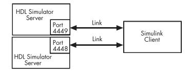
When you link the HDL simulator with a Simulink application, the simulator functions as the server. Using the EDA Simulator Link IN communications interface, an HDL Cosimulation block cosimulates a hardware component by applying input signals to and reading output signals from an HDL model under simulation in the HDL simulator.
