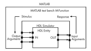
The following figure shows how a MATLAB component function is wrapped around by and communicates with the HDL simulator during a component simulation session.
